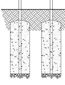
NOTE: CONCRETE FOOTING AND NO. 4 REBAR (BY OTHERS) PER LOCAL SOIL CONDITIONS. CONSULT PROJECT ENGINEER FOR EXACT REQUIREMENTS.
